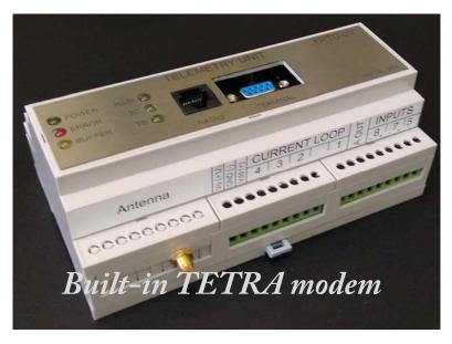
TRTU with built-in TETRA modem connects by I/O to external sensors (CURRENT LOOP), execution units (OUTPUTS) and dry contacts (INPUTS), audio notification system (A-OUT). It is configured to send TETRA SDS in hex from mobile and fixed installations now format to Data Base Applications and can be remote manageable. Inputs run high or low.
